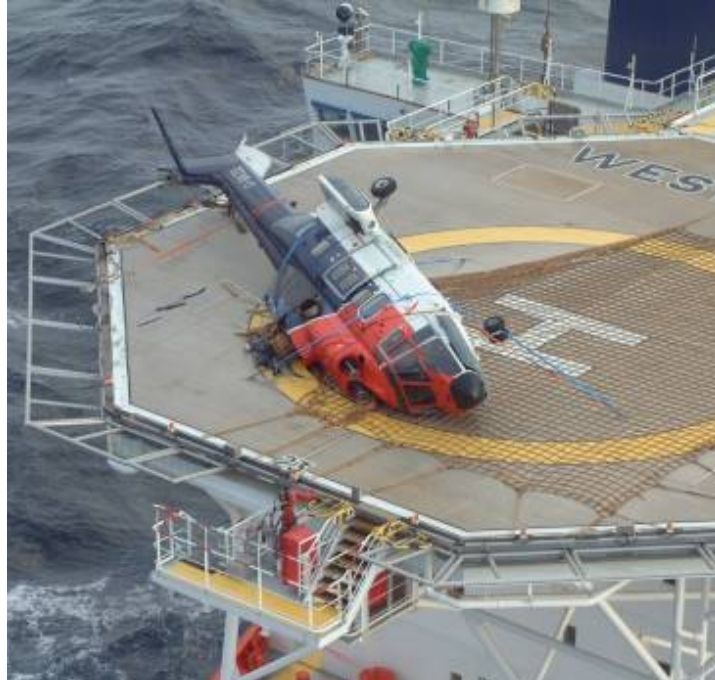
Figure 18: Super Puma rolled over on the West Navion drilling ship
