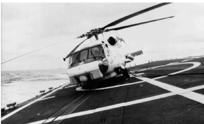
Figure 2. Typical shipboard securing condition
