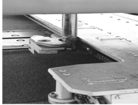
Figure 13: INDAL's passive ASIST securing system securing an intermediate-sized helicopter
