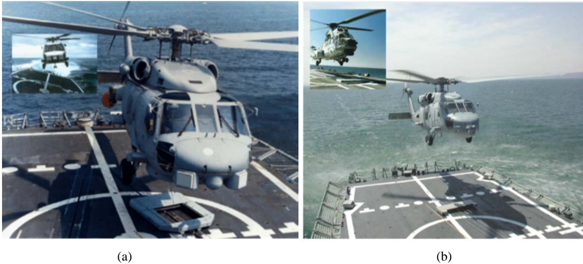
Figure 1: Helicopter landing on a moving platform with the aid of a) RAST and b) ASIST
