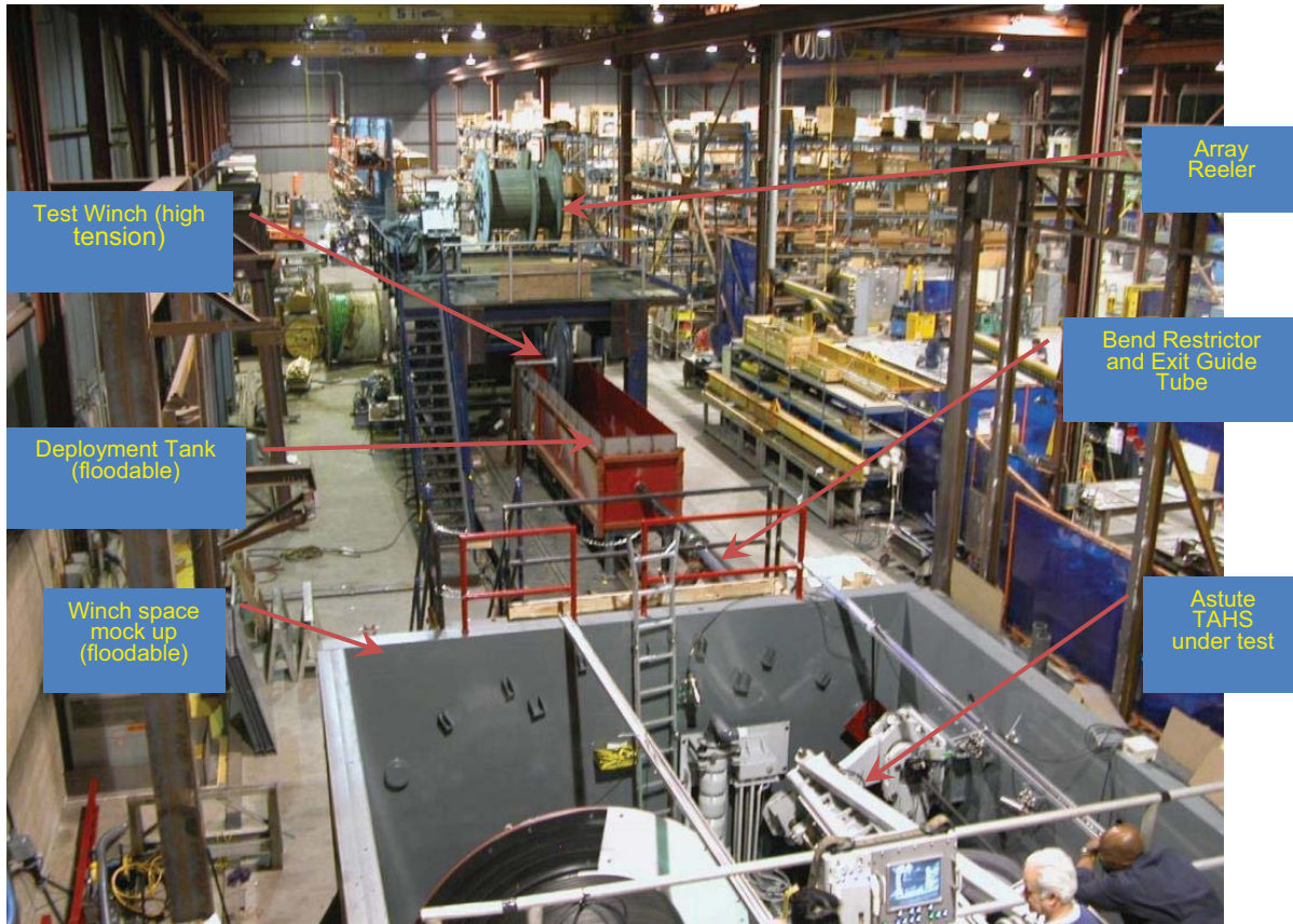
Figure 5: Astute TAHS under test at INDAL'S Facility
