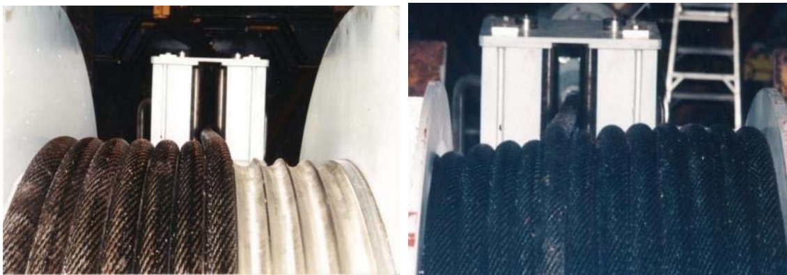
Figure 10: Parallel grooving first layer compared to seventh layer
