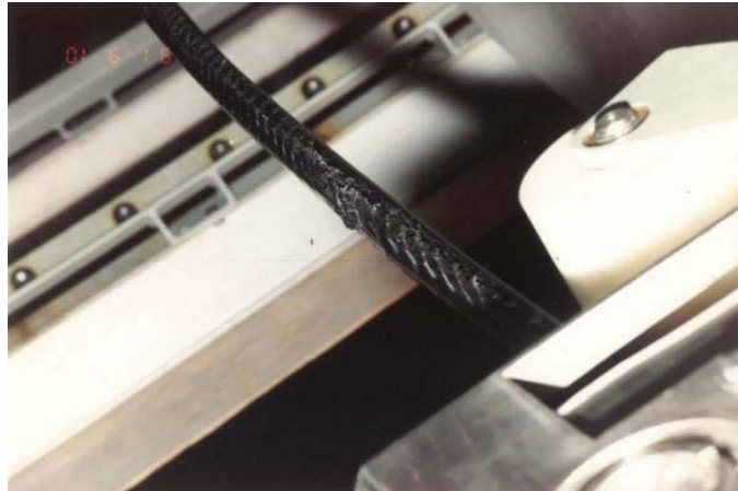
Figure 6: Jacket Damage Caused By Roller Contact
