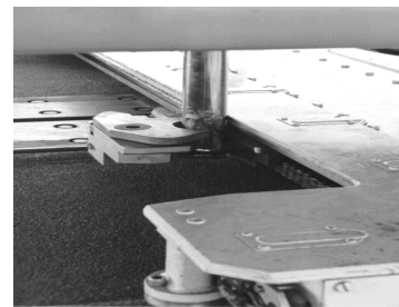
Figure 8: ITI's passive ASIST securing system securing an intermediate-sized helicopter
