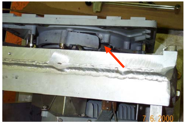
Figure 10. View of the aluminum upper flange indicating the expected mode of probe system fatigue failure
