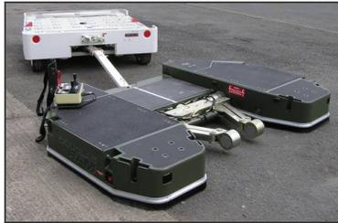
The tow pin adaptor can be utilised for towing trailers, weapon loading trolleys or any tow bar adapted unit
