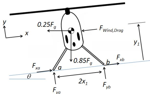
Figure 4: Quasi-static model of an unrestrained UAV
