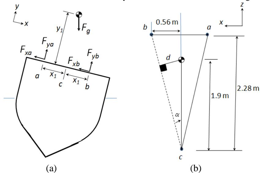
Figure 2: (a) UAV forces on rolled ship, (b) Elevation view of the UAV on-deck contact points (not to scale).
