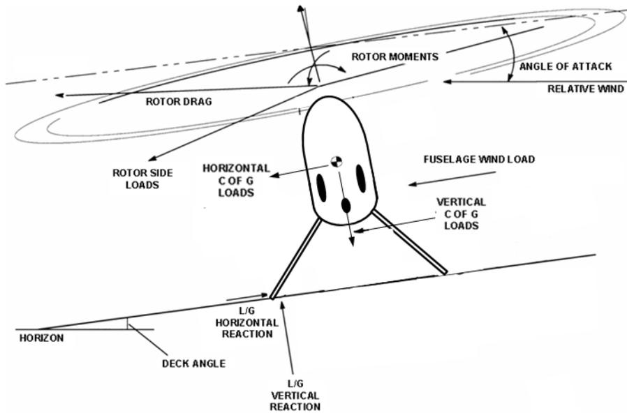
Figure 7: Load diagram of an unrestrained UAV on-deck
