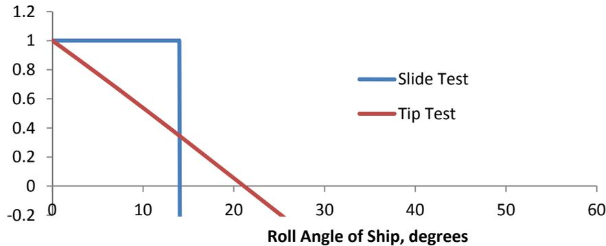
Figure 5: Stability of a UAV based on quasi-static analysis
