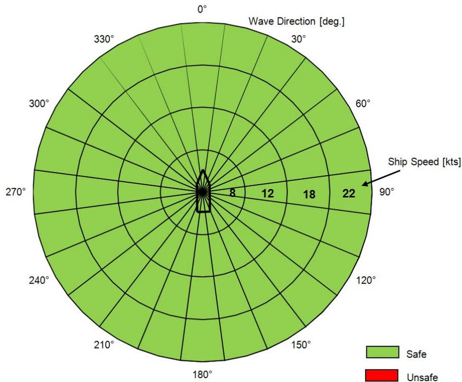
Figure 12: Safe and unsafe wave directions and corresponding ship speeds for a restrained UAV.
