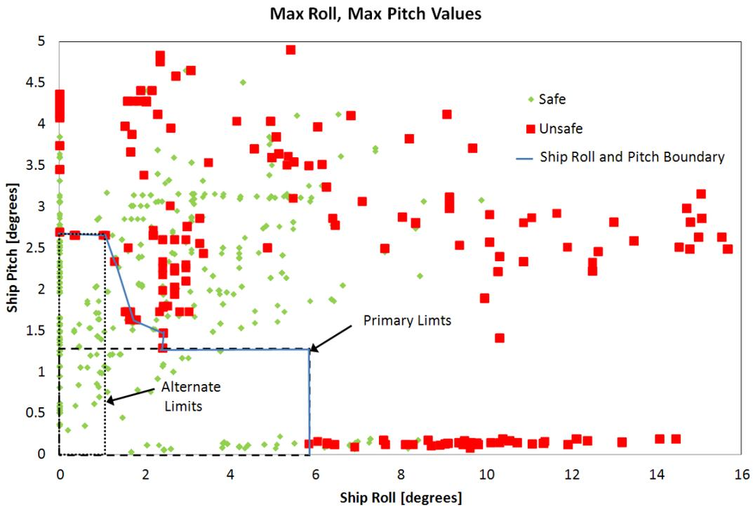
Figure 8: Maximum roll and maximum pitch values for an unrestrained UAV.
