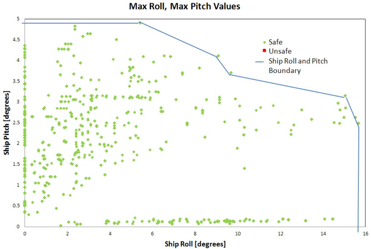
Figure 11: Maximum roll and maximum pitch values for a restrained UAV.
