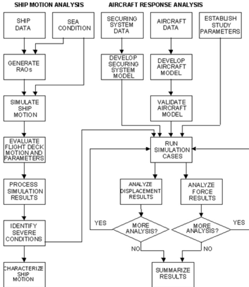
Figure 6: UAV/Ship time domain analysis procedure
