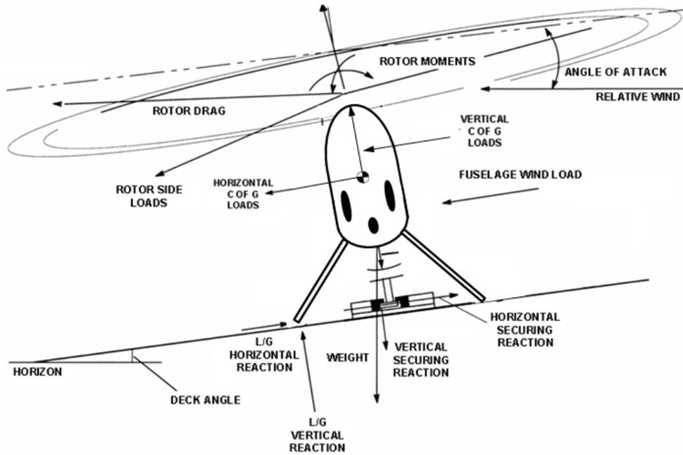
Figure 10: Load diagram of a restrained UAV on-deck
