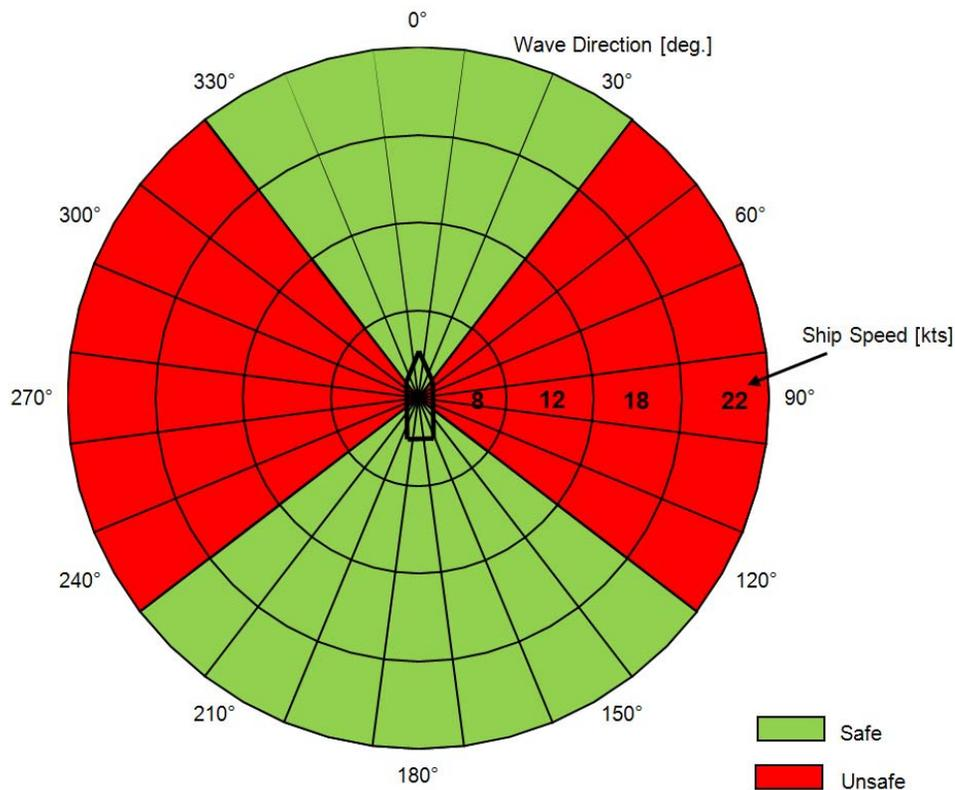
Figure 9: Safe and unsafe wave directions and corresponding ship speeds for an unrestrained UAV.
