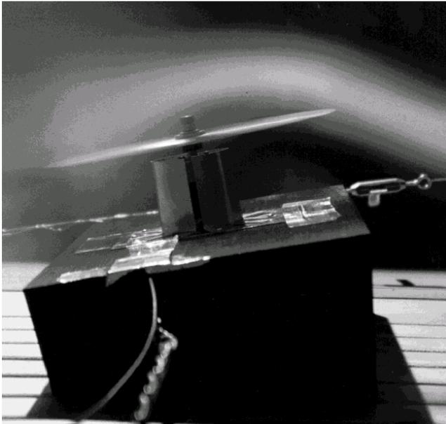
Figure 1: Rotor and deck model during wind tunnel testing
