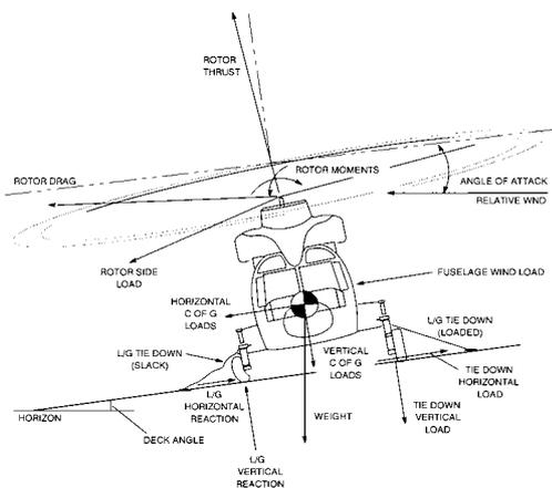
Figure 3: Loads acting on the embarked helicopter
