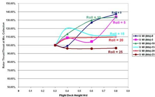
Figure 9: Effect of the deck height on the rotor thrust
