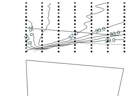
Figure 6 a: Time-averaged streamwise velocity contours for the 5° roll angle
