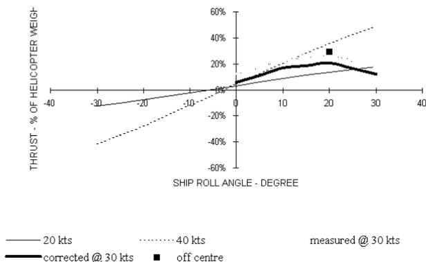
Figure 2: Rotor thrust from analytical model and from testing
