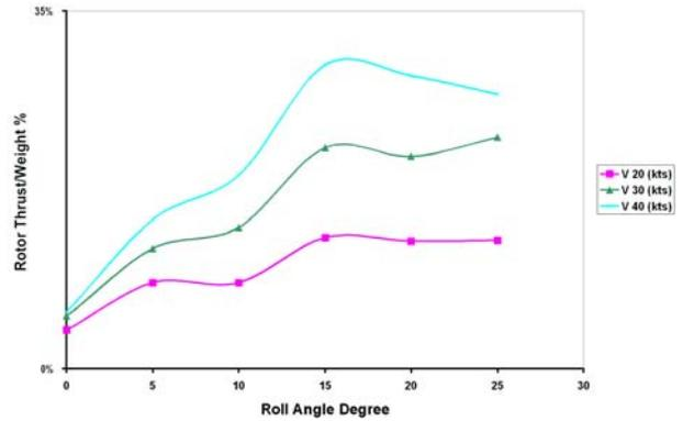
Figure 7: Effect of the roll angle on the rotor thrust
