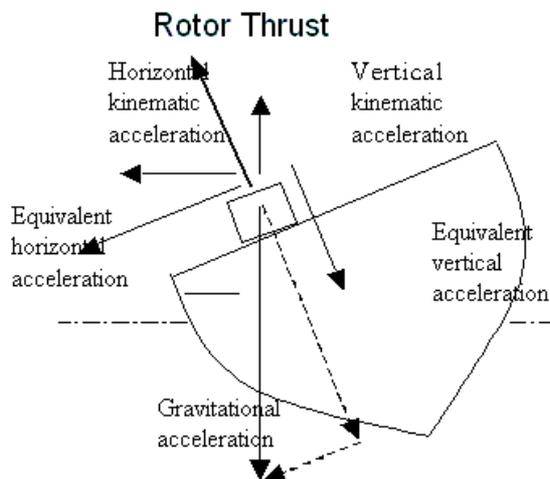
Figure 4: 2D representation of equivalent accelerations
