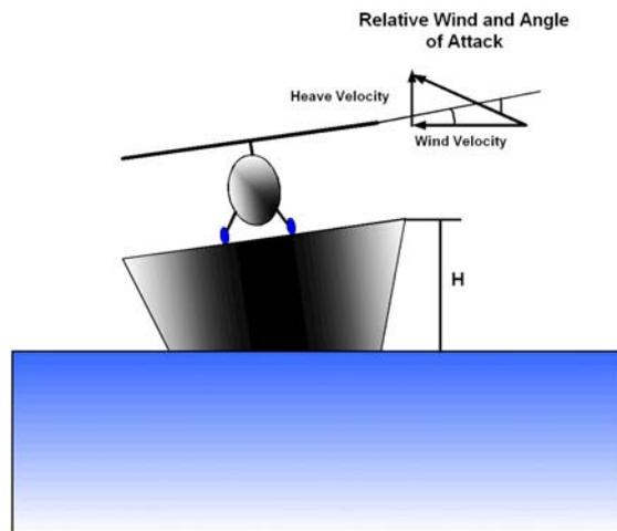
Figure 10: Heave Motion and Angle of Attack
