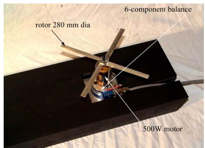
Figure 5: Rotor, electric motor, and balance mounted to the flight deck
