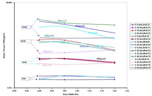
Figure 8: Effect of the deck width on the rotor thrust
