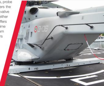
Once the aircraft has been secured, it is ready to be aligned for traversing to the hangar or any intermediate location. All deck handling operations can be accomplished without the need for personnel on the flight deck. TC-ASIST provides a secure and rapid straightening and traversing function with no personnel or cables on the deck.
